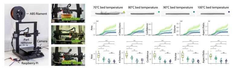
Warp severity predictions lead to autonomous correction and prevention of deformation
