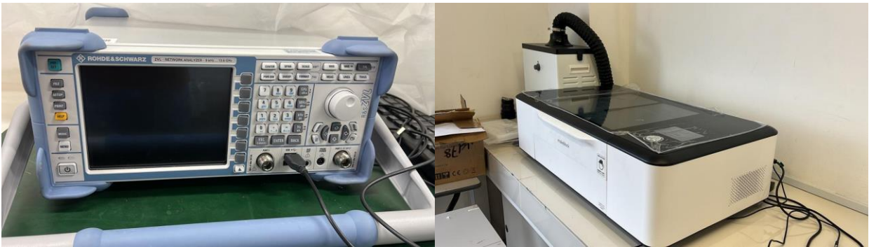
Picture 3: The Vector Network Analyzer; Picture 4: The antenna fabrication station
