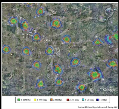
This is the first in a series of studies by EDX, showing uplink coverage for a well- designed network at 700MHz, compared to a network based on the same cell sites, but using 2600MHz.
