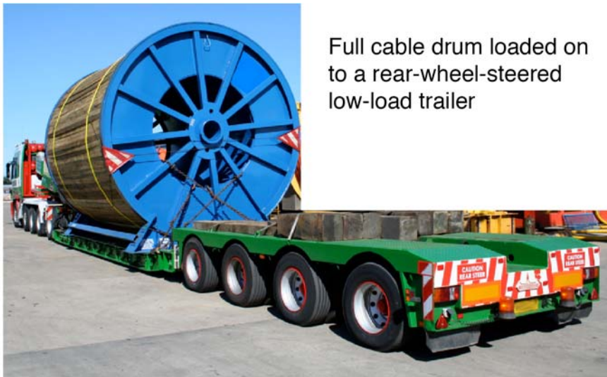
Figure 39 – Cable drum loaded transversely onto a trailer
