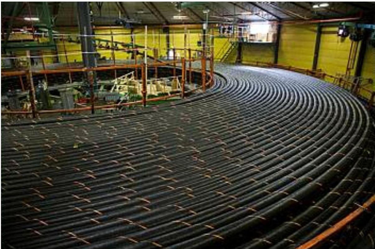
Figure 51 – Subsea cable on factory turntable.
