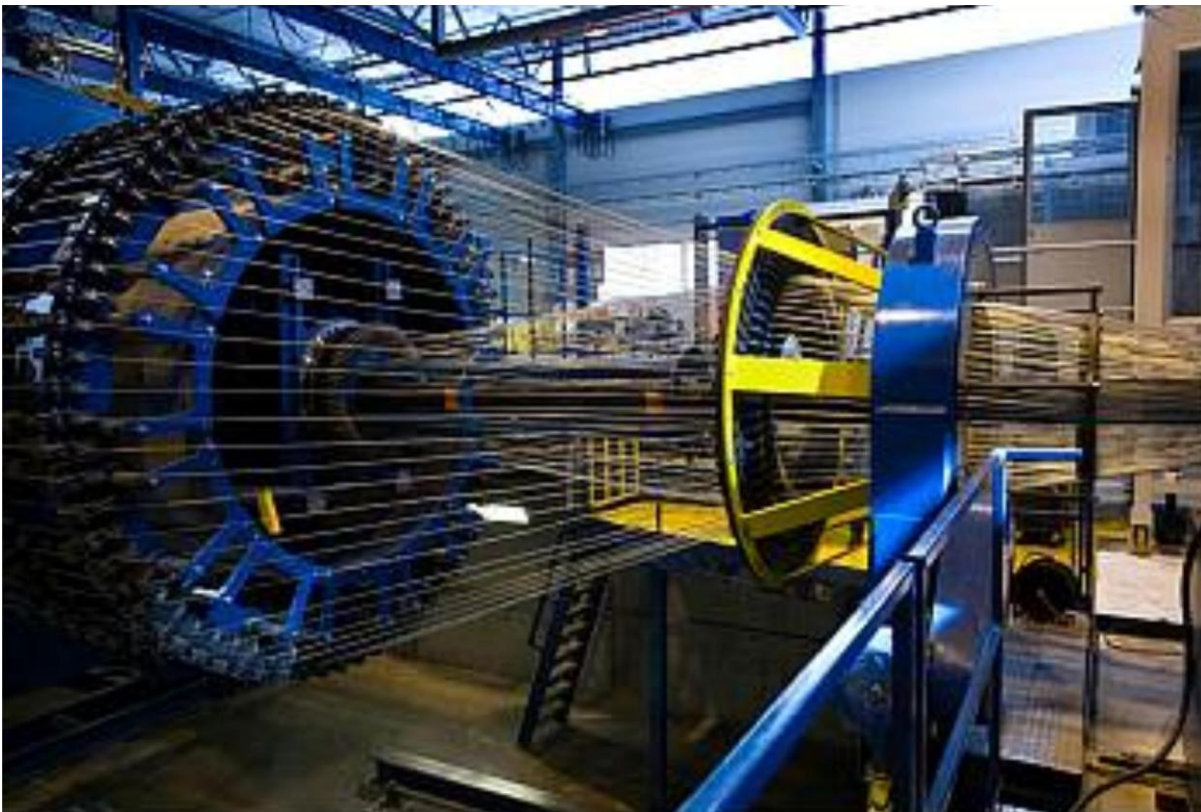
Figure 50 – Subsea cable armouring process
