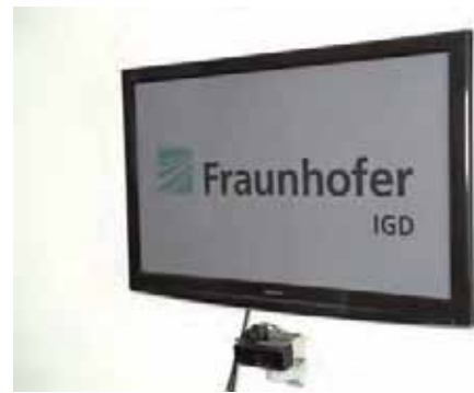
Figure 2 Display with uEye camera and Panasonic ToF range sensor mounted below
