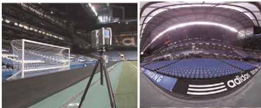
Figure 2 3D laser scanner (left), captured planar view (right)
