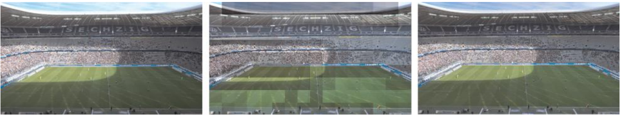
Figure 7 Left: Virtual aperture. Middle: Virtual aperture performed on 9×16 blocks. Right: Sectional tone mapping with z=0.25 .
