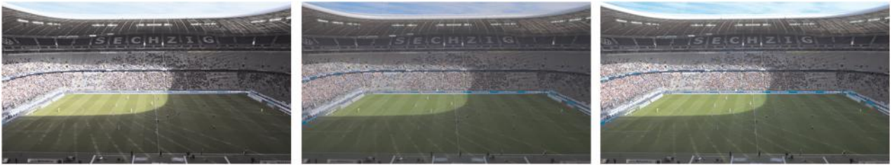
Figure 6 Left: A typical live broadcast situation shown with a camera transfer curve. Middle: The same situation shown with the Drago global tone mapping operator. Right: Using the virtual aperture with the Drago operator.
