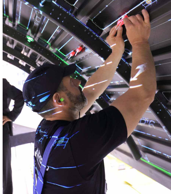
The MiRA application aiding production of an Airbus A350 XWB fuselage shell at the company's plant in Stade, Germany. (Source: Airbus).
